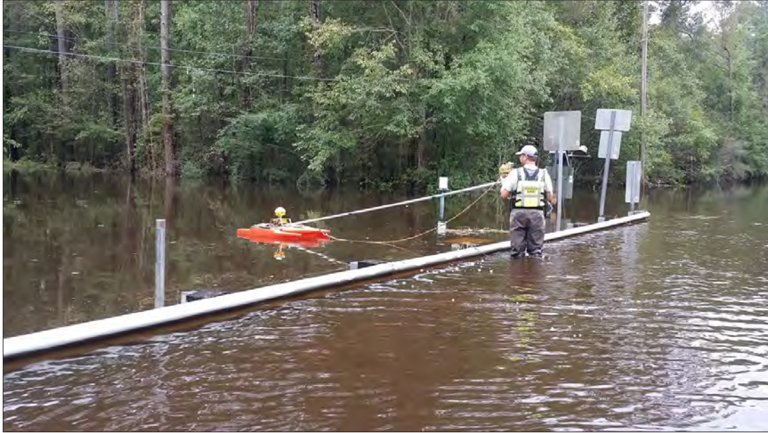
Figure 7. U.S. Geological Survey personnel making a streamflow measurement at station 02110701, Crabtree Swamp at Conway, South Carolina, using an acoustic Doppler current profiler.
