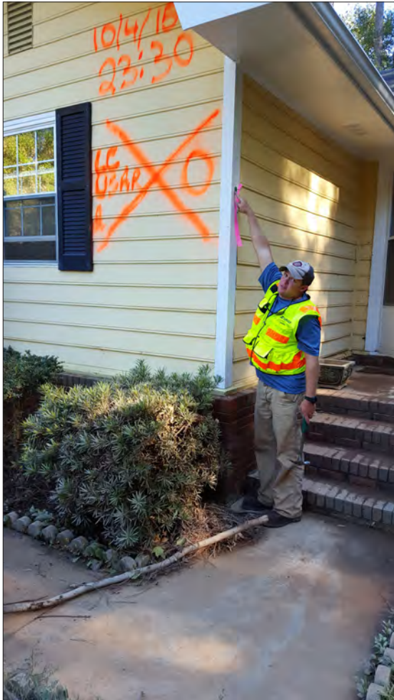
Figure 9. U.S. Geological Survey field crews conducting surveys of high-water marks to document the depth of flood waters in Lexington County, South Carolina, for the October 2015 flood.
