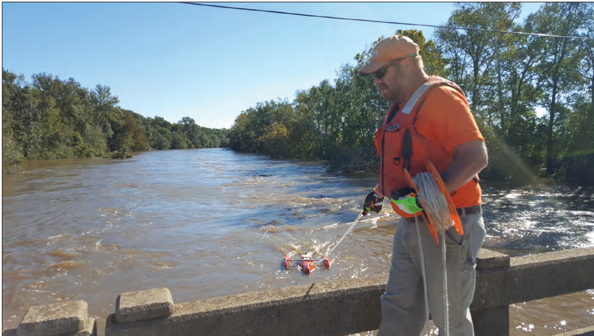
Figure 7. U.S. Geological Survey personnel using an acoustic Doppler current profiler to make a streamflow measurement at USGS station 02089000, Neuse River near Goldsboro in Wayne County, North Carolina, October 10, 2016. Photograph by John Mazurek, USGS.
