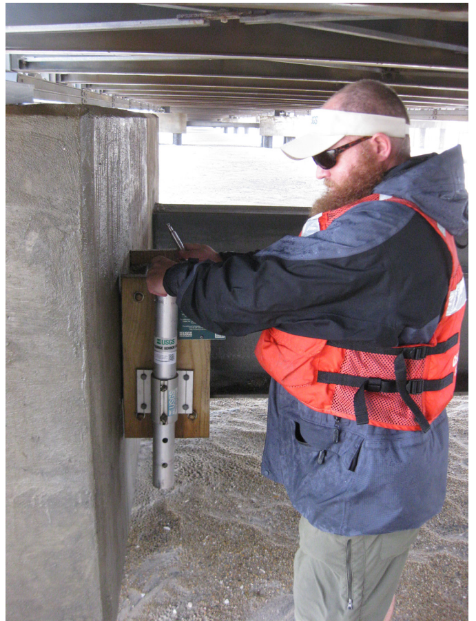
Figure 2. U.S. Geological Survey (USGS) scientist Ryan Rasmussen deploying a storm-tide sensor near Rodanthe, North Carolina, October 2016 (photograph credit: J. Curtis Weaver, USGS).
