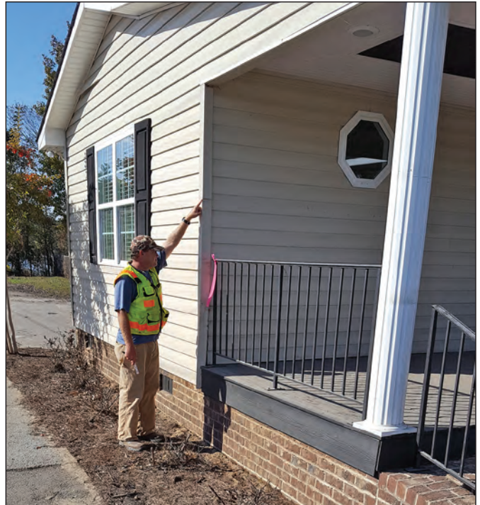
Figure 9. U.S. Geological Survey field crews conducting surveys of high-water marks to document the elevation of flood waters in Robeson County, North Carolina, for the October 2016 flood. This high-water mark identified on October 19, 2016, at a residence off LaClaire Road near Lumberton was measured at nearly 7 feet above the ground. Photograph by Jonathan J. Graham, USGS.
