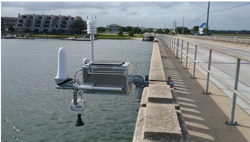
Figure 4. U.S. Geological Survey (USGS) rapid-deployment gage collecting real-time water-level and meteorological data at the Salisbury Street bridge leading to Wrightsville Beach, North Carolina, October 2016 (photograph credit: Shawn Spivey, USGS).
