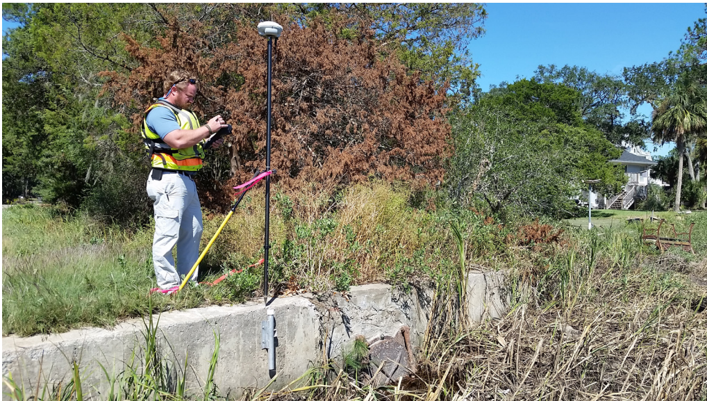
Figure 5. U.S. Geological Survey (USGS) scientist Jonathan Graham using a global positioning system to survey storm-tide elevation for Hurricane Matthew on Wilmington Island, Georgia, October 2016 (photograph credit: Arthur Day, USGS).
