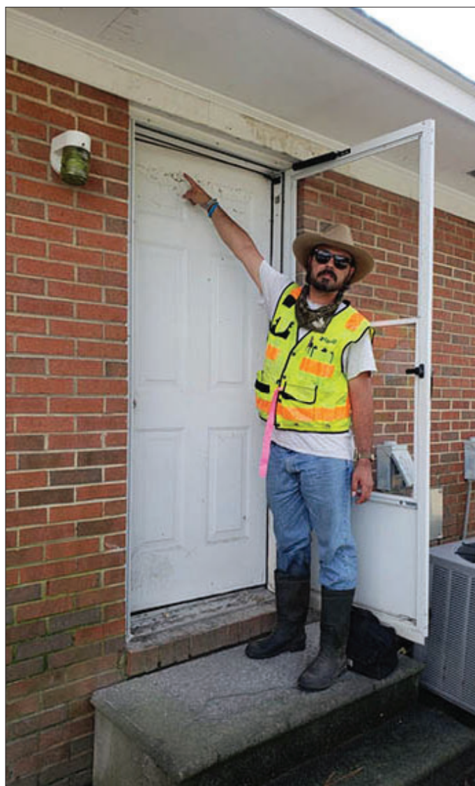
Figure 9. U.S. Geological Survey field crews conducting surveys of high-water marks to document the depth of flood waters near Northeast Creek in Piney Green in Onslow County, N.C., for the September 2018 flood.
