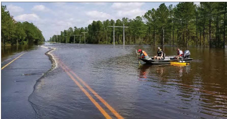
Figure 6. U.S. Geological Survey personnel use an acoustic Doppler current profiler to make a streamflow measurement of flood waters from the Cape Fear River in Kelly, North Carolina, on September 20, 2018.
