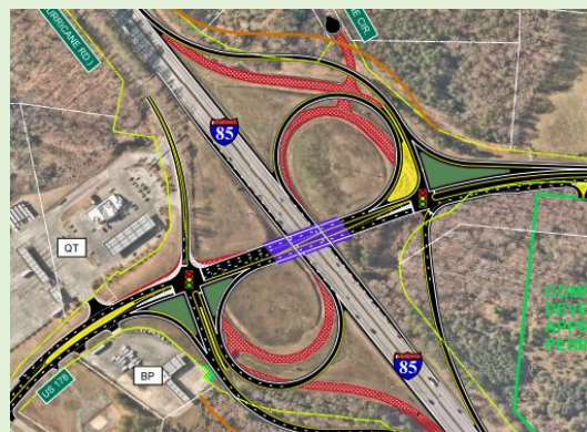
Alternative 2: Modified Partial Cloverleaf
